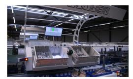
The choice was made to go for a shuttle system with three aisles with ten shuttles per aisle (thirty in total) which was supplied by Inther. "A shuttle system is the best fit within the contours of our premises. If so desired, we can have a fourth aisle with another ten shuttles placed next to it, "knows Van Es.
